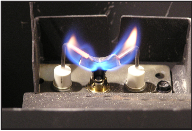
Figure 3.1 IPI Pilot Flame Patterns
